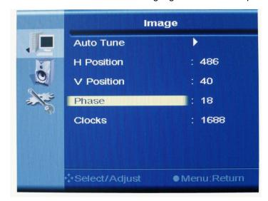
b. Press " $_{\triangle}$ " or " $_{\nabla}$ " to adjust the phase of signal. Then press "1" to confirm the adjustment and back to Image menu.
